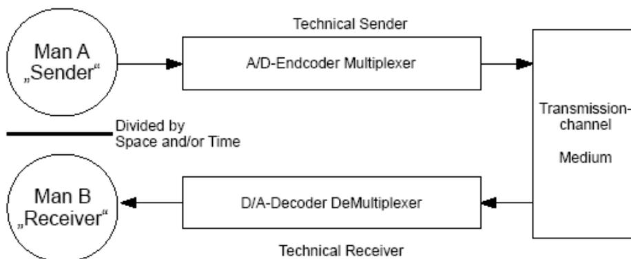
**Figure 2: Communications model over digital channel**
